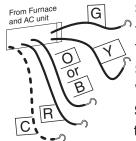
STEP 1 - Connect the **G** wire to the **G** terminal on the thermostat.
