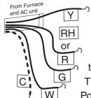
STEP 1 - Connect the Y wire to the Y terminal on the thermostat. This connects to the Cooler compressor. STEP 2 - Connect the RH or R wire to the RH terminal on the thermostat. This connects the Heater/Cooler Power.
