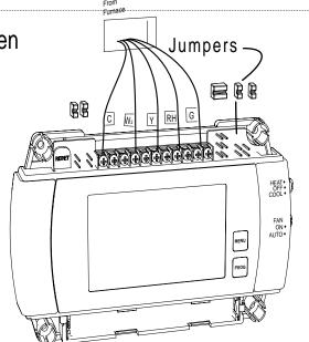
require you to find the 'other end' connection for each wire on your heating or air conditioning equipment and read the label there.
