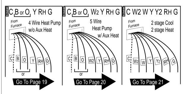
• If your combination of wires is not above you can use the wiring table on pages 24-25 to determine your connections, or call our USA support line at 1-877-505-2353 for help.
