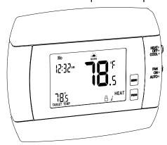
When using a heat pump with Auxiliary heat, if the heat pump cannot keep up and/or is defective, touch the MENU button, then touch PUMP; the PUMP OFF icon will come on.. The aux heat will then be your only source of heat. When the heat pump is again operational, be sure to turn the heat pump back on by touching MENU and then PUMP (off icon goes out) as the aux heat is more expensive than pump heat.
