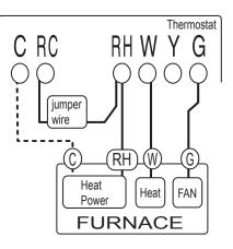
Your system is now conected to the thermostat. NOTE: Wires marked with the dotted line are optional.
