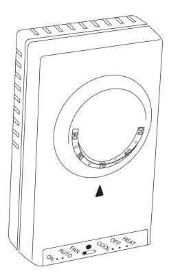
The 6008 can be used with most 24 volt gas, oil or electric heating and air conditioning systems, or gas millivolt heating systems. It cannot be used with 120 volt heating systems or heat pump systems. Ask The Home Depot for other thermostats to control those systems.
