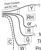
Y terminal on the thermostat. This connects to the Cooler compressor.
