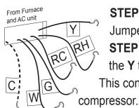
**STEP 1 -** Remove the orange Jumper wire.
