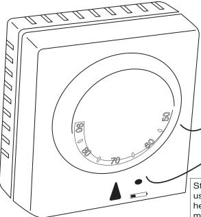
This unit is a "heating only" unit and cannot control a cooling system.
